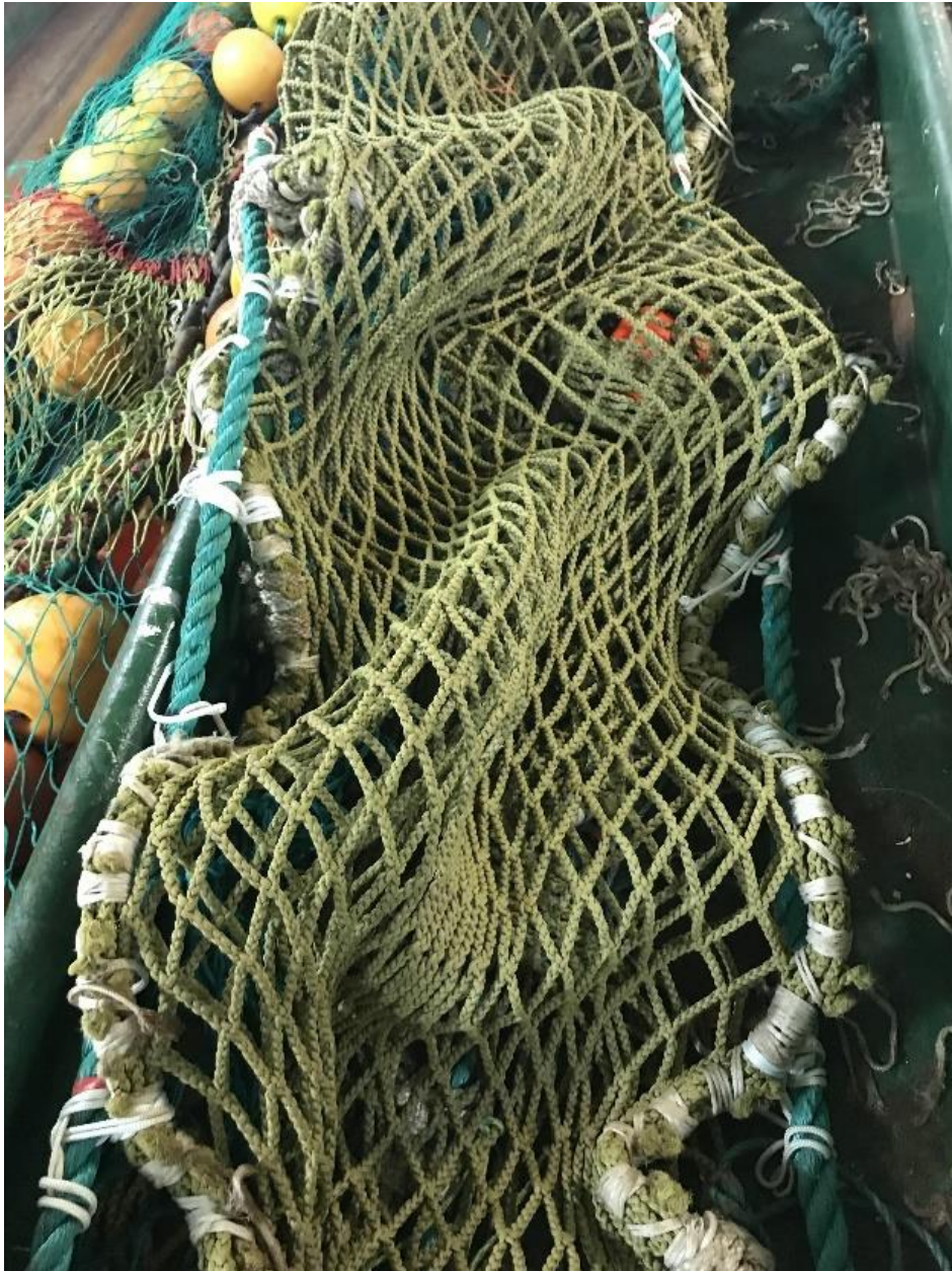
Fig. 5: Folding in a codend with SLR.
